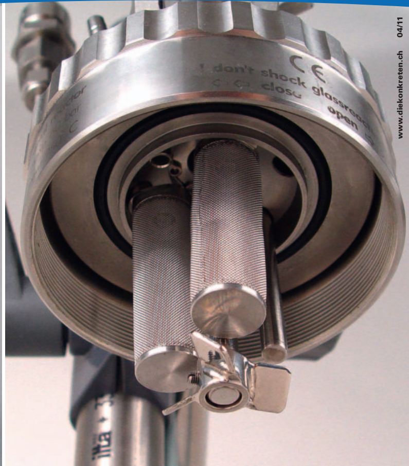
Double fixed catalyst basket with increased interaction surface for 200ml / 10 bar glass reactor
