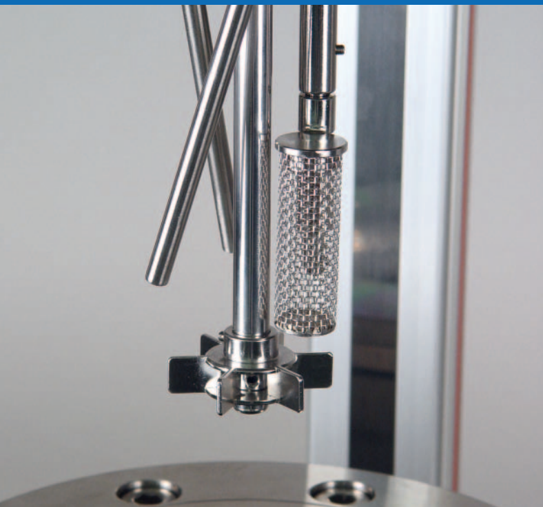
Fixed catalyst basket and turbine stirrer with gassing stirrer shaft for 1 liter / 60 bar reactor
