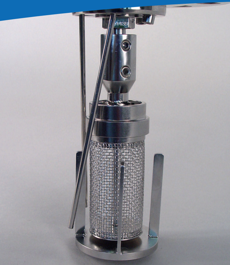
Spinning catalyst basket for 300ml / 350 bar reactor
