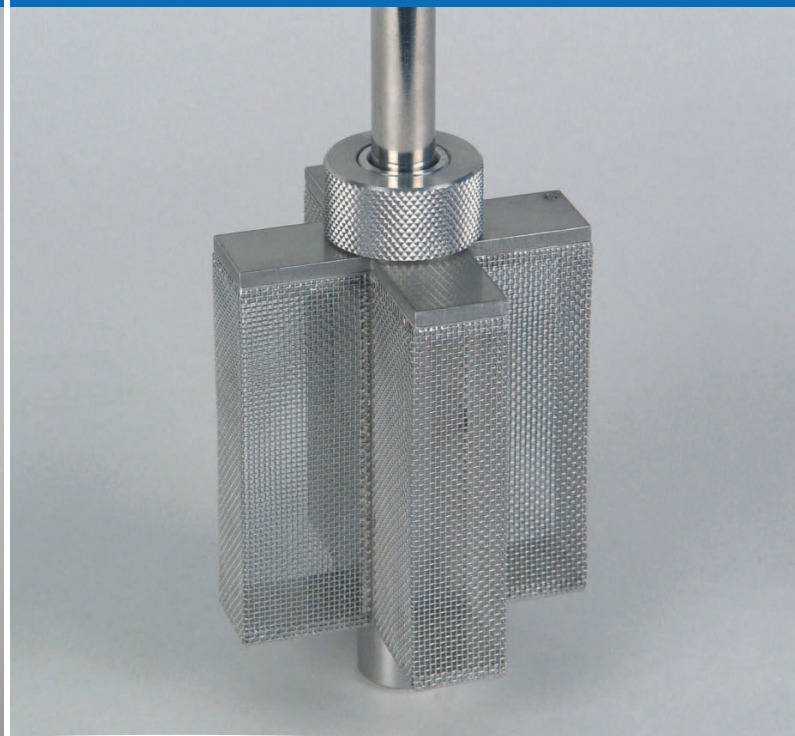
Spinning catalyst basket for 3 liter / 200 bar reactor
